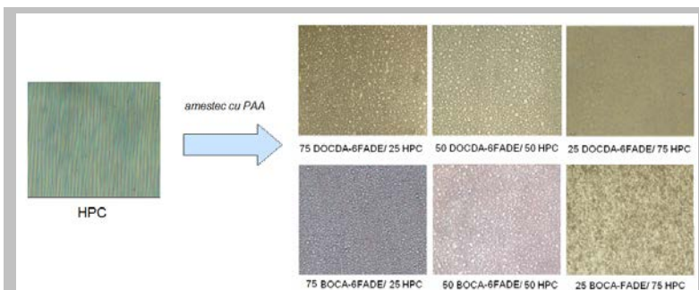
Figure 9. Images of polarized light microscopy of HPC and of the mixtures in various reports with the two PI precursors
